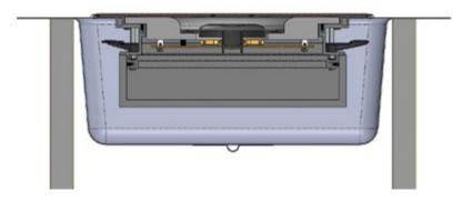
40mm ceramic fiber insulation Overall size: 478 x 482 mm
