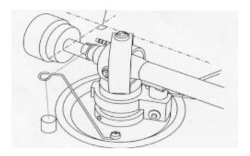
**11.** Slide the dust cover (20) onto the dust cover hinges (15) on the back of the plinth. If necessary, adjust the tightness of the hinges by turning the dust cover hinge screws (16).
