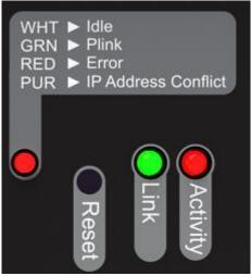
The Pixelator Mini comes with one RGB status LED and two green network LED indicators located on the right side of the front panel
