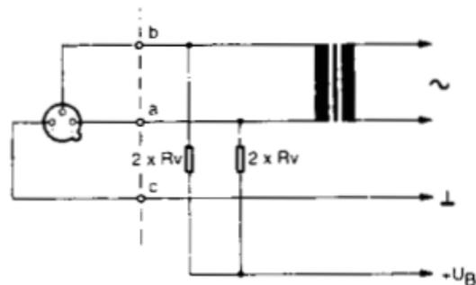
3. In case where single ended (grounded) amplifier inputs, or where no input transformers are available, either capacitors or optional transformers have to be wired into the audio lines to prevent any current leakage into the input circuitry.
